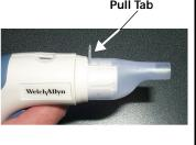
Plastic flow limiter must be in place for all aerators. See page 4 in manual.
