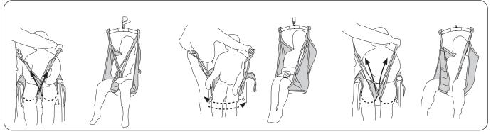
**Crossed-over leg supports.** The most common way of applying the sling. One leg support loop is passed through the other before the loops are connected to the sling bar. **Overlapped under both thighs.** This can be appropriate, for example when lifting a patient with amputated legs. **Note:** In order to avoid the patient's sitting posture being too reclined, Extension Loops can be attached to the leg support loops. Each leg support connected separately to the sling bar.
