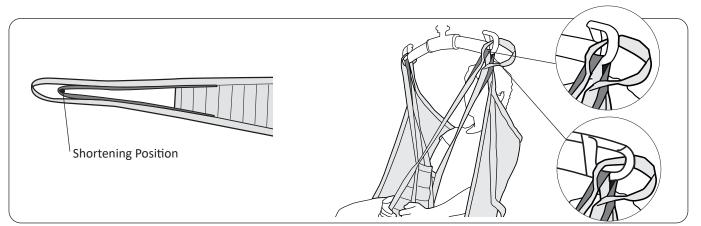
Our sling is carefully designed to ensure that the patient always sits with pressure well distributed between legs and back section for good support during transfers. However, in certain cases it can be preferable to use the inner setting, the "shortening position", on the leg support loop to change the patient's sitting position.
