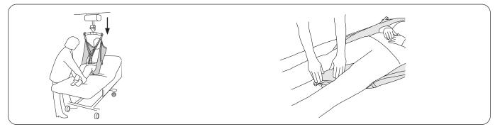
Position the patient above the bed. Raise the head end of the bed for the patient's comfort. Lower the patient onto the bed. Lower the head end. Place the leg support loops under the leg supports between the patient's legs.
