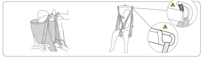
**Note:** Check that all suspension loops have the same length, i.e., are at an equal height when they are stretched prior to lifting. Adjust the position of the sling if they are not at an equal height.
